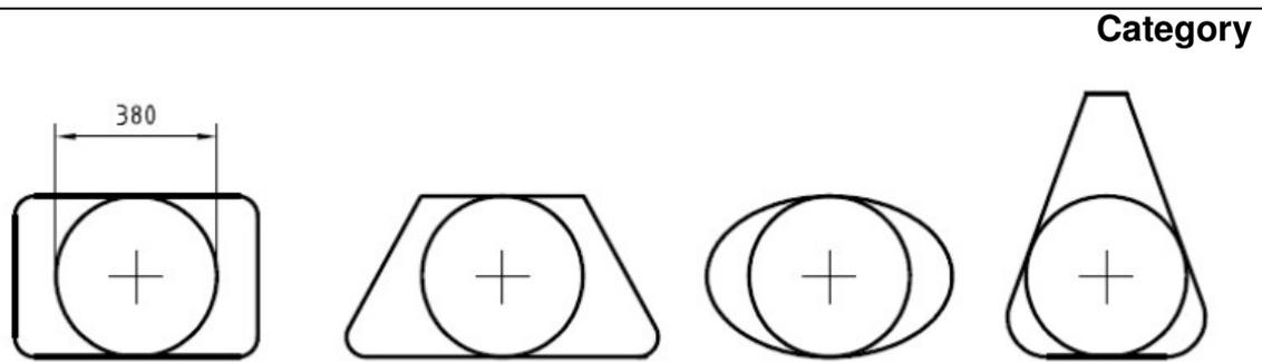
Figure 1 - Measurements of Minimum Clear Opening
